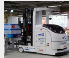
Autonomous forklift Receiving, dispatching
