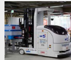
Autonomous forklift Receiving, dispatching
